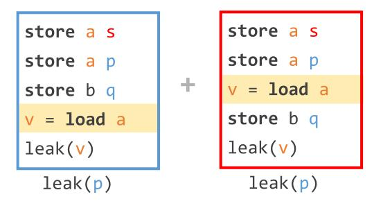
**Spectre-STL:** Loads can speculatively bypass prior stores
