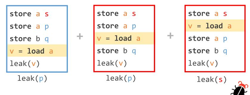
**Spectre-STL:** Loads can speculatively bypass prior stores
