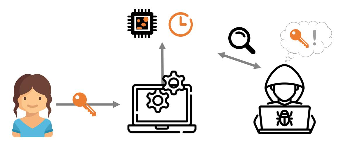
*Timing and microarchitectural attacks can be run remotely* [1]
