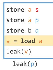
**Spectre-STL:** Loads can speculatively bypass prior stores
